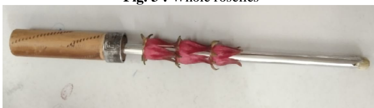
Plate 4 : The tool fabricates to detached seed from whole roselles
